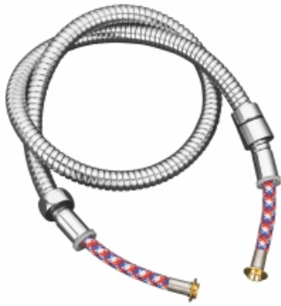
High Pressure SS304 CP Shower Tube with Nylon Coated Inner Hose Pipe DG-ESS-213 - 1 Mtr. DG-ESS-214 - 1½ Mtr. Working Pressure : 15 Bar
